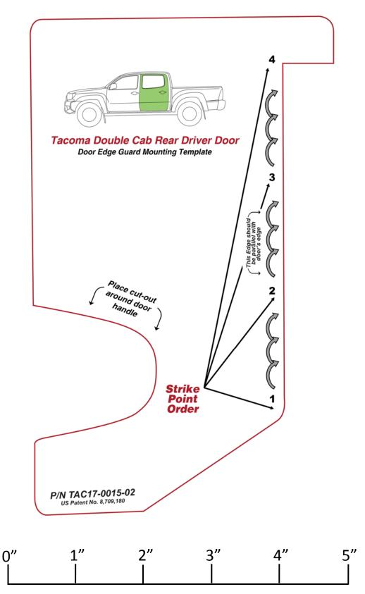
Dealer Installation Note: Check the above scale to ensure it is 1:1. Adjust on photocopier if it is not to scale. If this is a pdf document, set the "Page Scaling" to "None" in the Print dialogue box prior to printing.
